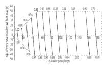
· Correction ratio for heating capacity
