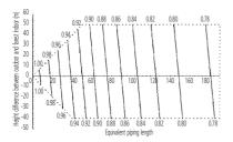
Correction ratio for heating capacity
