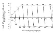
Correction ratio for heating capacity
